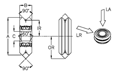
Diameter A = 19.58Hole size C = 4.76Internal radius IR = 7.95Outer radius OR = 11.89Width B = 7.87
